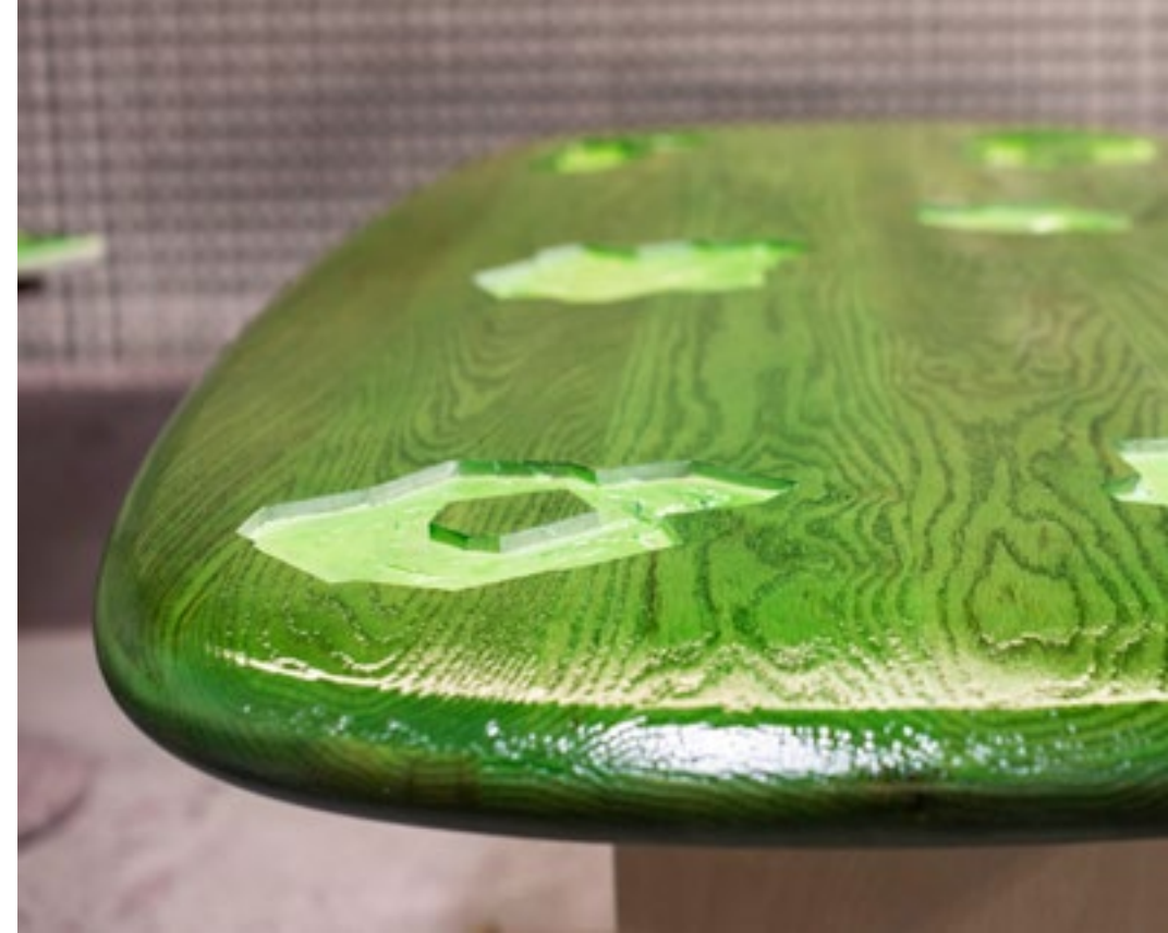
A green, epoxy resin coating protects the red oak tabletop from the elements, and the slight camber of the top encourages drainage from the surface.
