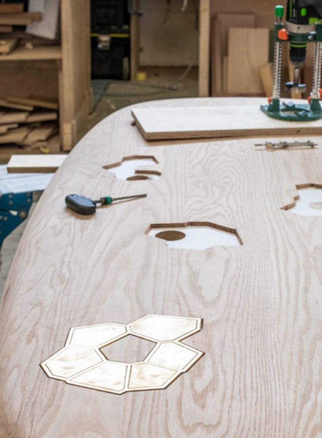
Hexagonal brass inlays mirror the random rock formations of the Giant's Causeway, doubling as covers for water drainage holes.
