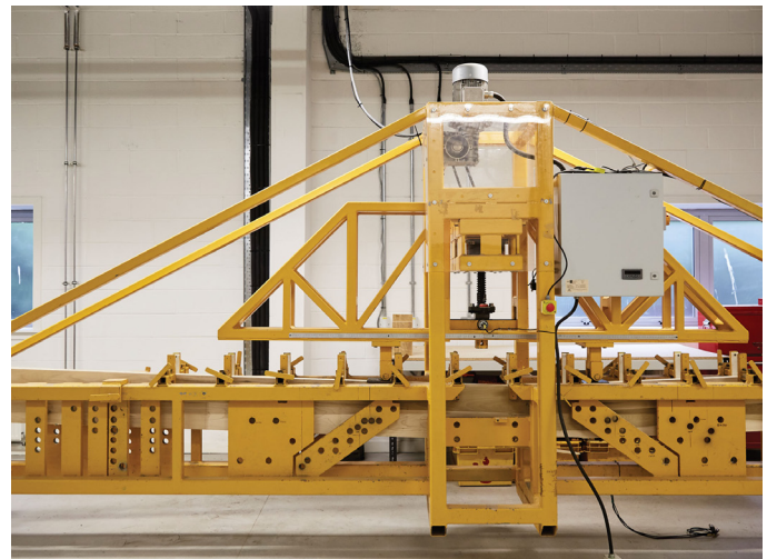
Edgewise bending testing at Edinburgh Napier University
