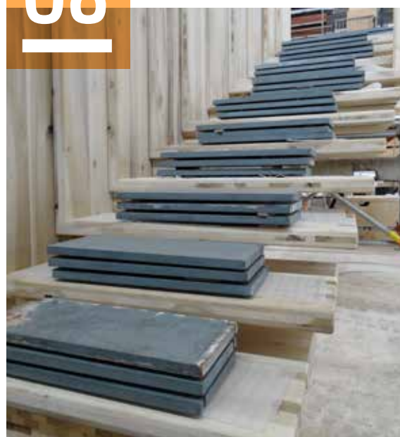
Test flight, loaded to simulate occupation in use.
