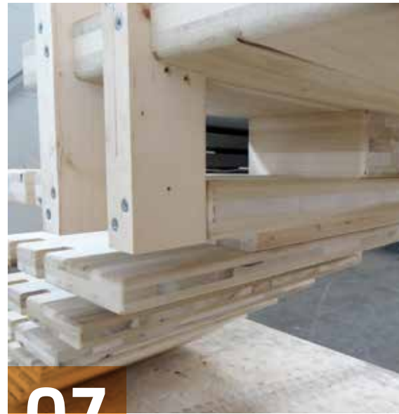
The test flight assembled, complete with balustrade posts which for the other flights were fixed on site.
