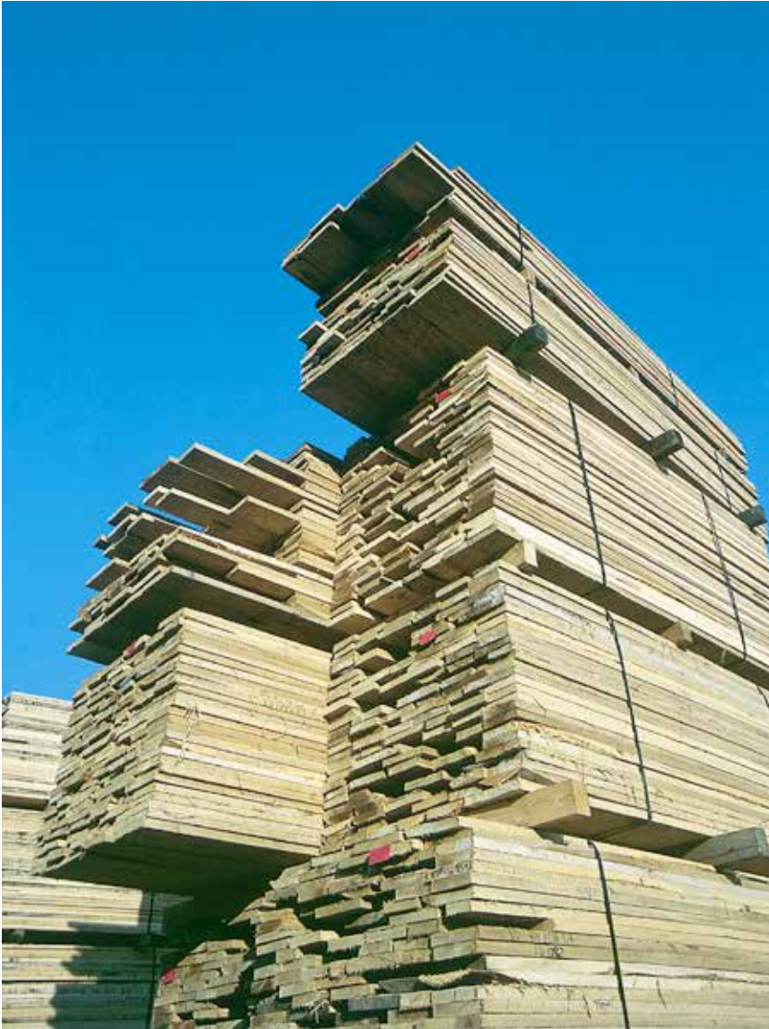
FIG 2 American sawmills cut timber in random widths and lengths, which may pose a challenge for traditional CLT manufacturers.
